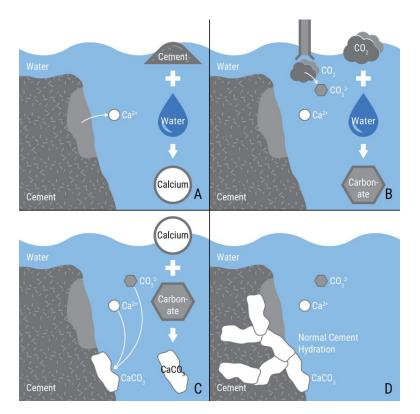
Figure 6. Example of a direct  $CO_2$  utilization process: a) water is added to cement leading to dissolution; b)  $CO_2$  is introduced and enters solution; c) solid phase calcium carbonate (CaCO<sub>3</sub>) is formed; d) normal cement hydration occurs with CaCO<sub>3</sub> acting as a nucleating agent<sup>49</sup>
